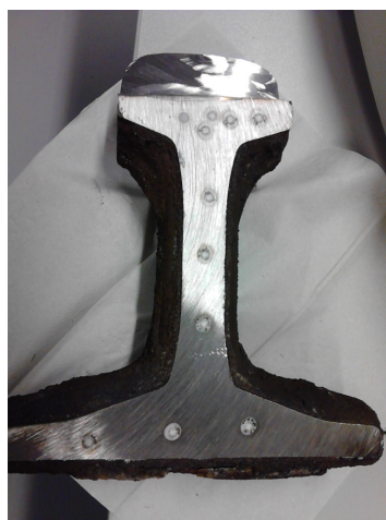
Fig. 5. Determination of chemical composition of ground exothermic welding joint: head, web, base
